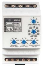
Apply three-phase voltage. The LED indicator should initially flash GREEN if in the Automatic Reset mode while the relay goes through its start-up delay or waiting for an external switch to be operated if in the Manual Reset mode
