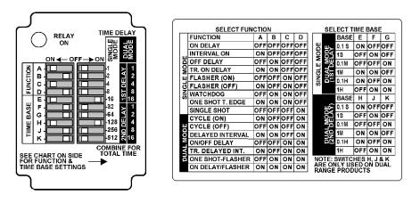
switch is marked with a binary time increment. The required delay is selected by moving the switch of each increment to the ON position & adding their corresponding values (see right). Note that dual mode products can either have the same or different ON & OFF times.
