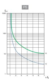
**Cold curve:** represents the performance of the relay without any previous current flow, first start.
