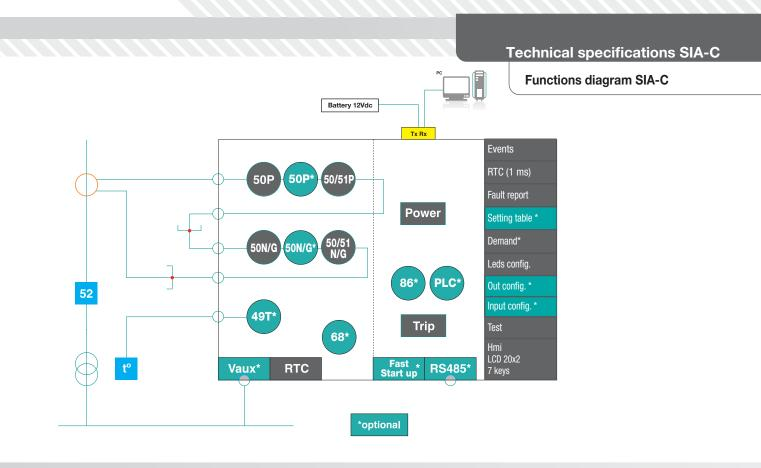
3 CT power supply-measurement 1 CT sensitive neutral Striker **Connections diagram SIA-C**
