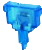
Diode plugs, blue - DSBL with 400 Volt 1A diode - cathode on the high rail side - the diode plugs are designed to prevent incorrect insertion.
