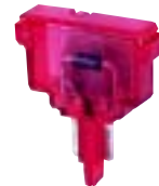
Diode plugs, red - DSRT with 400 Volt 1A diode - cathode on the low rail side - the diode plugs are designed to prevent incorrect insertion.
