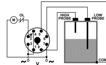
If the container is non-conductive or insulated, an additional probe must be installed as the COM connection where it will always be submerged.
